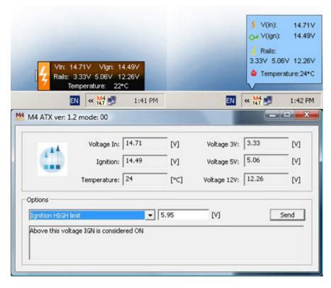
When you connect M4-ATX-HV by USB with your PC, then you can control voltages and temperatures with the control software. With the Advanced software version you even are able to change the behavior of the power supply.
